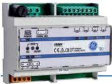
DIN-rail module, suitable for controlling four analog dimmers operating with input voltages of 0-10V or 1-10V (can be selected via HabiTEQ System Manager software). The control contains four digital-analogue converters with 8-bit precision.
