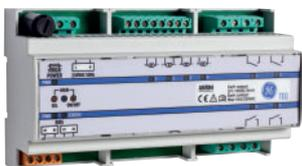
DIN-rail module, suitable for controlling four analog dimmers operating with input voltages of 0-10V or 1-10V (can be selected via HabiTEQ System Manager software). The control contains four digital-analogue converters with 8-bit precision.
