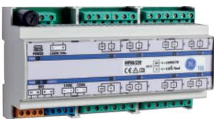
DIN-rail module for connecting external contacts such as solar/wind detector, motion detector, door switches and push buttons. There are 8 optically insulated inputs. Each input needs a voltage to be active. This can be:
